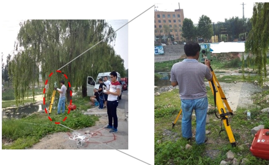
Fig. 10. Channel cross-sections measured by the Total Station method.
